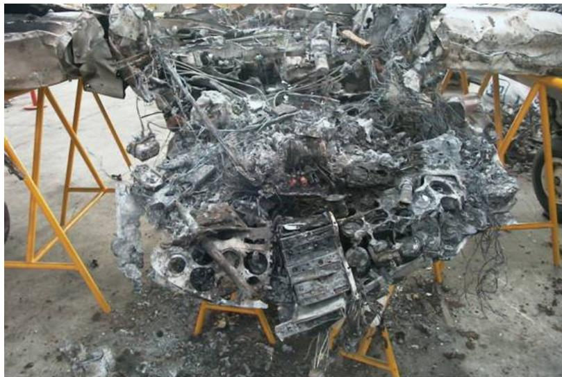
**Figure 2. Fire damage to cockpit and avionics**
